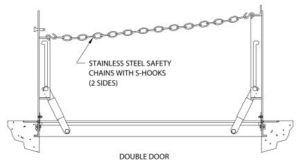
A safety barrier shall be provided on two accessible sides of the hatch when the doors are in the open position. The barrier shall consist of two lengths of 3/16 inch diameter stainless steel welded loop chain which are attached by stainless steel S-hooks to the opposing outward corners of each door leaf.
