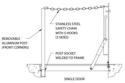
A safety barrier shall be provided on three accessible sides of the hatch when the door is in the open position. The barrier shall consist of three lengths of 3/16 inch diameter stainless steel welded loop chain which are attached by stainless steel S-hooks to two removable aluminum posts in the front corners of the hatch frame as well as to the outward corners of the door leaf.
